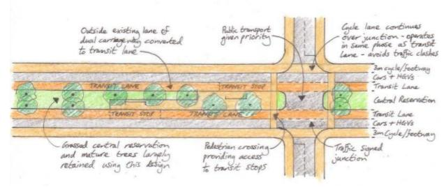
In addition, to suit the central reservation transit stops, the transit vehicles will need to be fitted with doors on both sides of the vehicle (as a tram or train) so that stops on either the left or right of the vehicle can be accommodated. This will give much more flexibility and require less road engineering works to make transit stops work with the existing highway and urban constraints.
